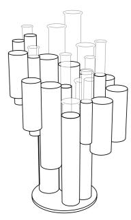
6. Slide the test tubes into the PVC tube with 22mm dia.
