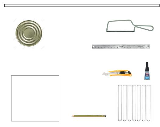
Matt white PVC Pipe, 40mm, 35mm,22mm dia. Tin Can with around 130mm dia. Handsaw, Ruler, Cutter, Superglue Foam Board, Pencil, Glass Test tube,
